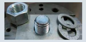
After disassembly, impression marks must be visible on both the fastener and the contact surface.
