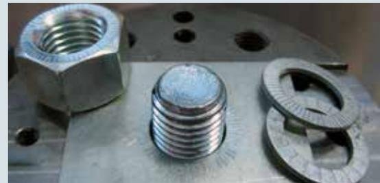
*After disassembly, impression marks must be visible on both the fastener and the contact surface.*
