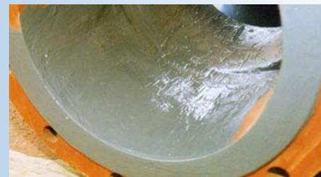
*The daily repair routine when epoxy-ceramic compounds are brush applied. No hydraulic engineer wants to see irregular surfaces like this . . .*
