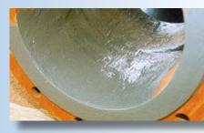
The daily repair routine when epoxyceramic compounds are brush applied. No hydraulic engineer wants to see irregular surfaces like this . . .
